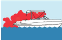
Exhaust gas trapped in enclosed places.
