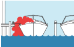
Blocked exhaust outlets.
