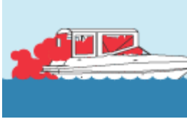
Inadequately ventilated canvas enclosures.
