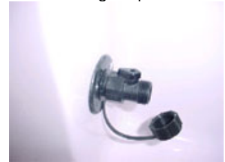
Lever on the washdown fitting is open
