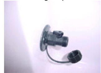
Lever on the washdown fitting is open
