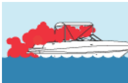
Exhaust gas trapped in enclosed places.
