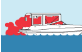
Inadequately ventilated canvas enclosures.
