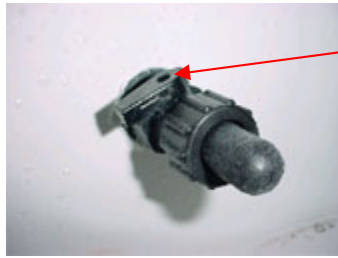
Lever on the aerator fitting is closed
