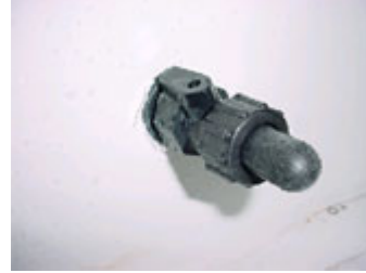
Lever on the aerator fitting is open
