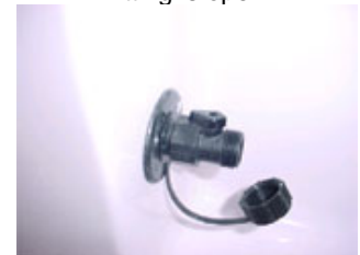
Lever on the washdown fitting is open
