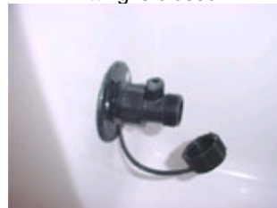
Lever on the washdown fitting is closed
