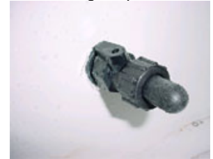
Lever on the aerator fitting is open
