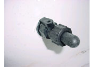
Lever on the aerator fitting is open
