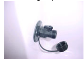
Lever on the washdown fitting is open
