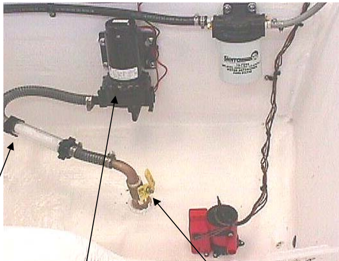
Raw Water Filter, Baitwell/Washdown Pump, Sea-cock (shown in the open position)
