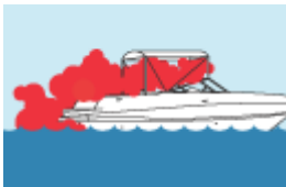
Exhaust gas trapped in enclosed places.
