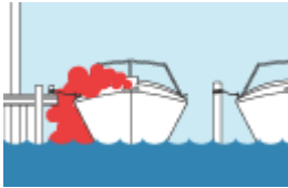
Blocked exhaust outlets.
