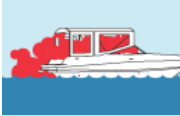
Inadequately ventilated canvas enclosures.
