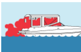
Inadequately ventilated canvas enclosures.
