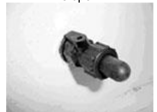
Lever on the aerator fitting is open
