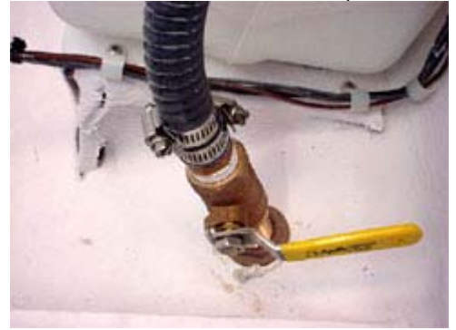
Seacock is shown in the closed position
