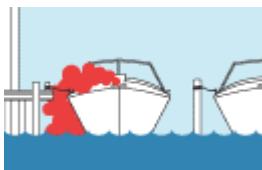
Blocked exhaust outlets.
