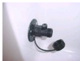
Lever on the washdown fitting is closed
