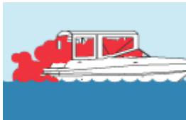
Inadequately ventilated canvas enclosures.
