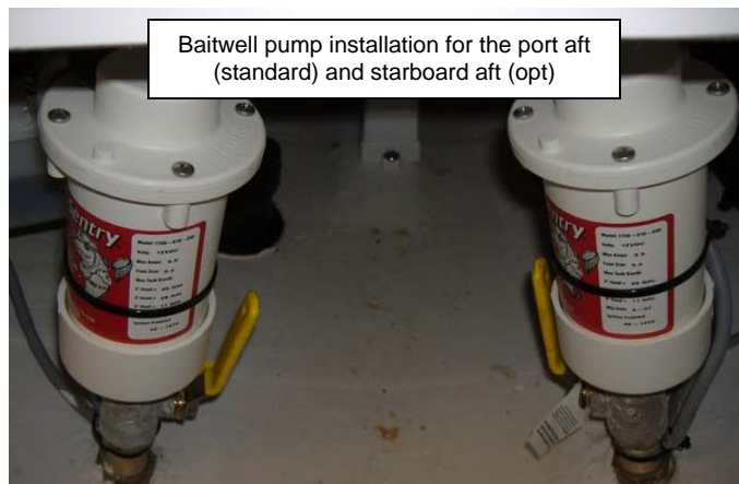
Lever on the aerator fitting is open
