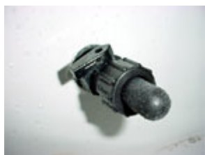
Lever on the aerator fitting is closed
