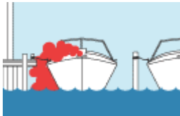
Blocked exhaust outlets.
