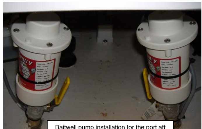
Baitwell pump installation for the port aft (standard) and starboard aft (opt)
