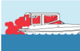
Inadequately ventilated canvas enclosures.
