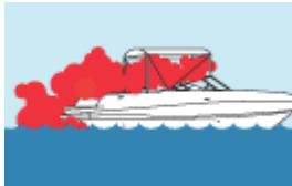
Exhaust gas trapped in enclosed places.
