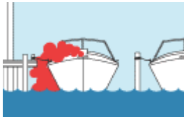
Blocked exhaust outlets.
