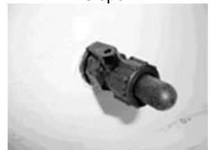
Lever on the aerator fitting is open
