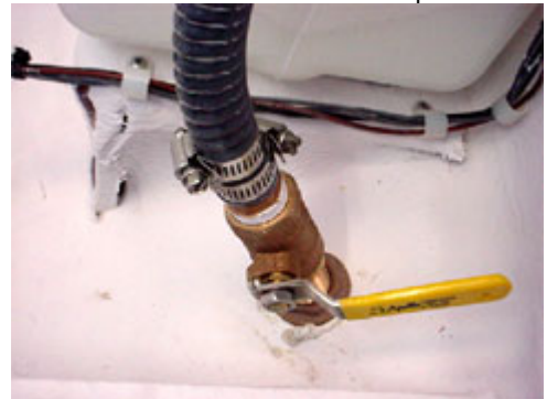
Seacock is shown in the closed position.
