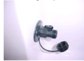
Lever on the washdown fitting is open
