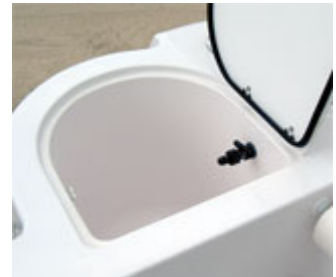
Seacock is shown in the closed position.
