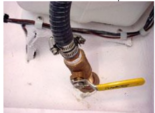
Seacock is shown in the closed position.
