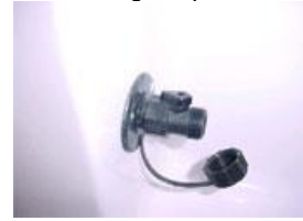
Lever on the washdown fitting is open
