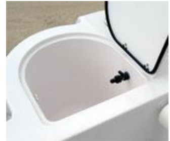
Seacock is shown in the closed position.
