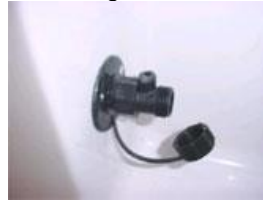
Lever on the washdown fitting is closed
