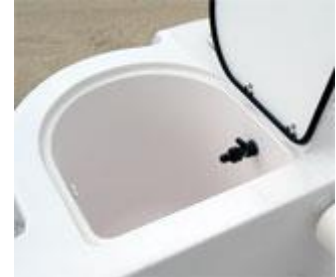
Seacock is shown in the closed position.
