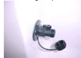
Lever on the washdown fitting is open
