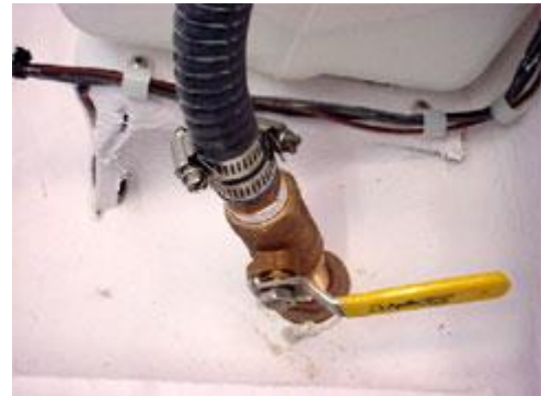
Seacock is shown in the closed position.
