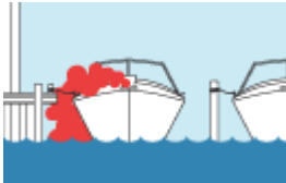
Blocked exhaust outlets.
