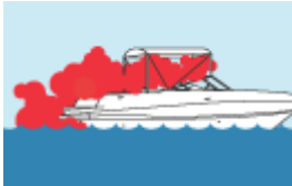
Exhaust gas trapped in enclosed places.
