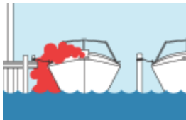
Blocked exhaust outlets.
