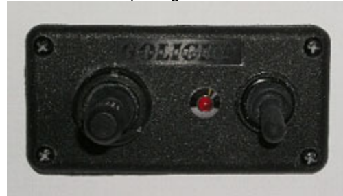
Remote Spot Light Control Panel
