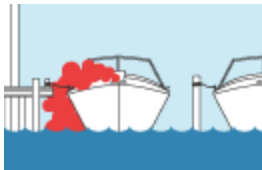
Blocked exhaust outlets.
