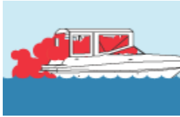
Inadequately ventilated canvas enclosures.
