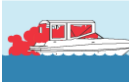
Inadequately ventilated canvas enclosures.
