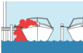
Blocked exhaust outlets.
