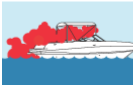
Exhaust gas trapped in enclosed places.
