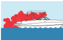
Exhaust gas trapped in enclosed places.
