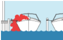
Blocked exhaust outlets.
