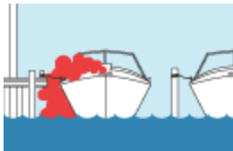
Blocked exhaust outlets.
