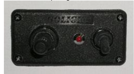
Remote Spot Light Control Panel
