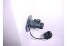
Lever on the washdown fitting is open
