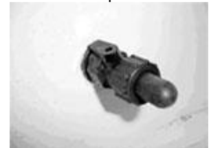
Lever on the aerator fitting is open
