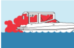
Inadequately ventilated canvas enclosures.
