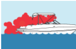
Exhaust gas trapped in enclosed places.
