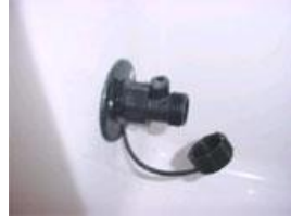
Lever on the washdown fitting is closed
