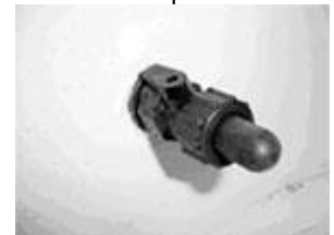
Lever on the aerator fitting is open
