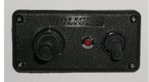
Remote Spot Light Control Panel
