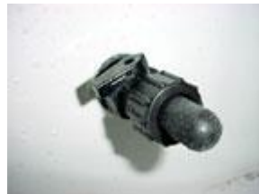
Lever on the aerator fitting is closed
