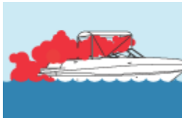
Exhaust gas trapped in enclosed places.
