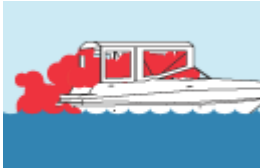
Inadequately ventilated canvas enclosures.
