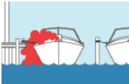
Blocked exhaust outlets.
