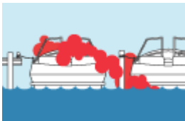
Another vessel's exhaust. CO from the boat docked next to you can be just as deadly.
