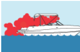
Exhaust gas trapped in enclosed places.
