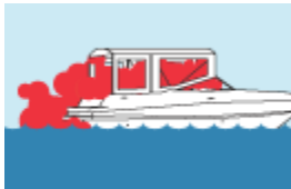
Inadequately ventilated canvas enclosures.
