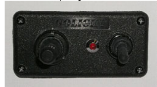
Remote Spot Light Control Panel
