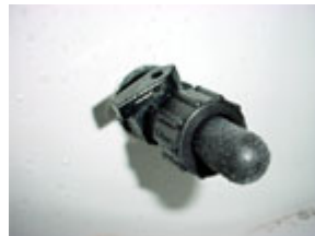
Lever on the aerator fitting is closed
