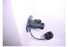
Lever on the washdown fitting is open
