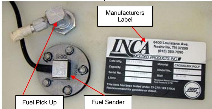
Located below the access pie installed forward of the helm seat and aft of the console.
