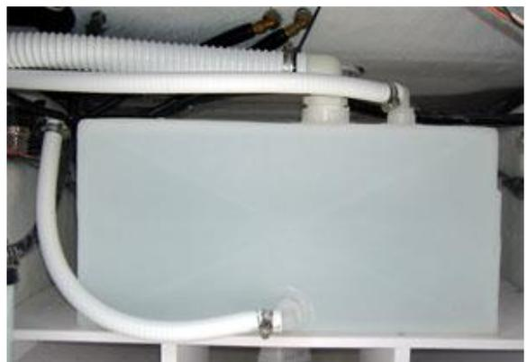
Important: Fill the tank with potable water only. Refilling the tank often will help to keep it a source of clean fresh drinking water. Never fill the fresh water tank with anything other than fresh water.
