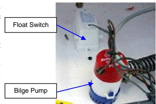
If for some reason the indicator light on your bilge pump switch comes on, check your bilge for water. It is not uncommon for rain water or water from washing your boat to accumulate in the bilge. Standing water will activate the automatic float that is connected to the bilge pump. If you notice your pump running frequently during your day on the water, you should check the thru hull fittings, hose connections, etc. for any possible leaks.
