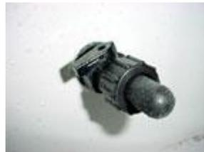
Lever on the aerator fitting is open
