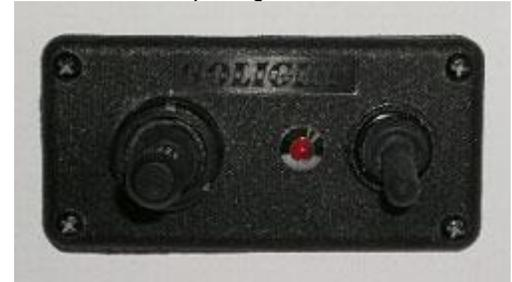
The switch on the right side of the panel allows you to turn the light on and off. The red LED light located in the center of the panel will be lit when the spot light is turned on. Once the spot light is turned on, the all around toggle lever (on the left side of the panel) can be moved in an up, down, left or right position to rotate the light assembly in the desired direction.
