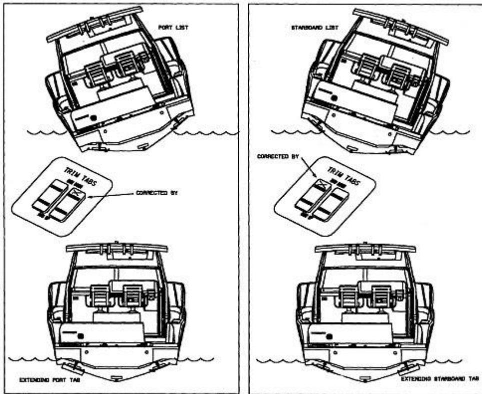
Warning: Trim tabs can cause a dramatic change in the attitude and heading of your boat. Adjust them in small increments when in open water and clear of any obstructions.
