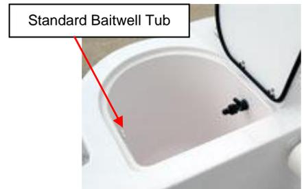
To operate the washdown system: Locate the baitwell switch on the console and press the switch to the forward position to turn on the baitwell/washdown pump. Then, locate the black washdown fitting at port aft corner of the cockpit.
