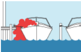
Blocked exhaust outlets.
