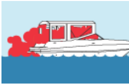
Inadequately ventilated canvas enclosures.
