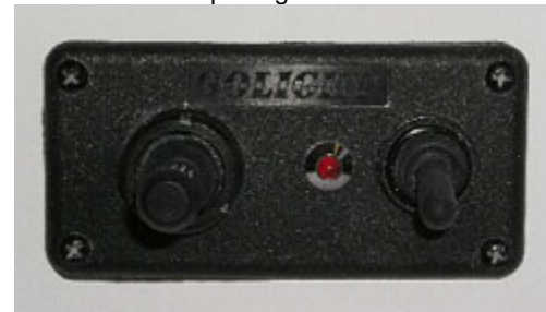
Remote Spot Light Control Panel
