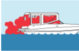
Inadequately ventilated canvas enclosures.
