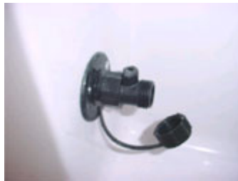
Lever on the washdown fitting is closed
