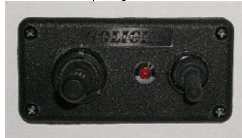
Remote Spot Light Control Panel
