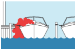
Blocked exhaust outlets.
