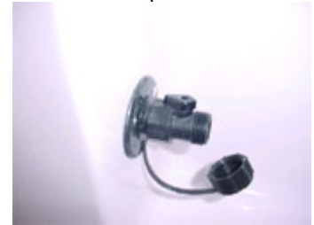
Lever on the washdown fitting is open
