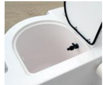
Lever on the washdown fitting is open
