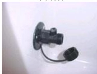
Lever on the washdown fitting is closed
