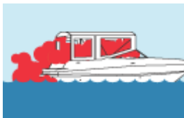
Inadequately ventilated canvas enclosures.
