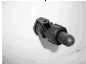
Lever on the aerator fitting is open
