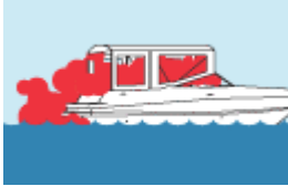
Inadequately ventilated canvas enclosures.
