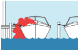
Blocked exhaust outlets.
