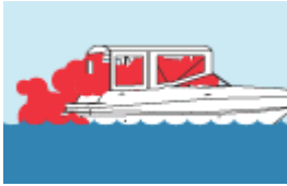
Inadequately ventilated canvas enclosures.
