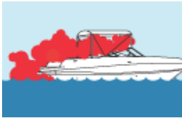
Exhaust gas trapped in enclosed places.
