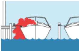
Blocked exhaust outlets.
