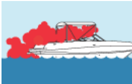
Exhaust gas trapped in enclosed places.
