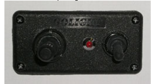
Remote Spot Light Control Panel
