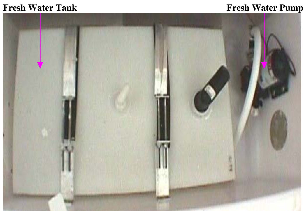
<fig. 6 – Fresh Water System>
