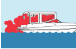
Inadequately ventilated canvas enclosures.
