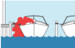
Blocked exhaust outlets.
