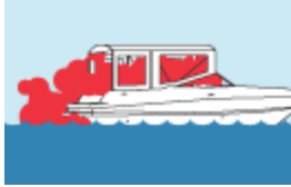
Inadequately ventilated canvas enclosures.
