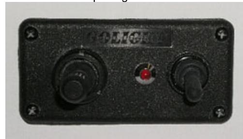
Remote Spot Light Control Panel
