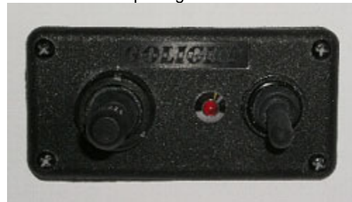
Remote Spot Light Control Panel
