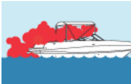
Exhaust gas trapped in enclosed places.
