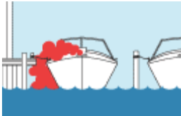
Blocked exhaust outlets.
