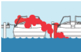
Another vessel's exhaust. CO from the boat docked next to you can be just as deadly.
