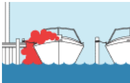
Blocked exhaust outlets.
