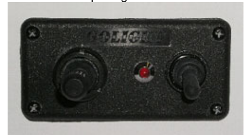
Remote Spot Light Control Panel
