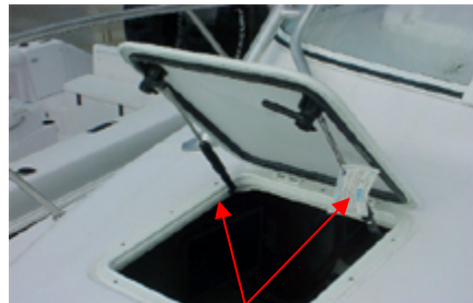
There is a black plastic cylinder on each mounting arm.
