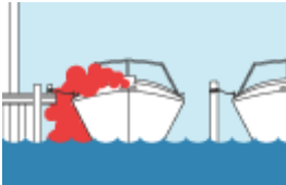
Blocked exhaust outlets.
