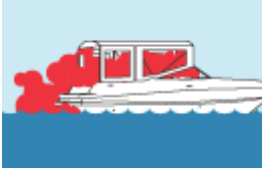
Inadequately ventilated canvas enclosures.
